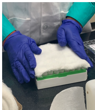
Pack cryobox with absorbent material (cotton roll/ tissue paper)
