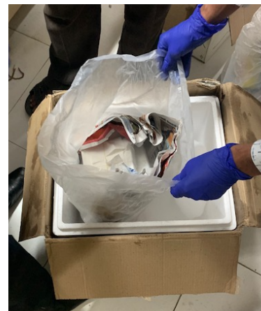
Place cryobox in bag with dry ice inside thermocol
